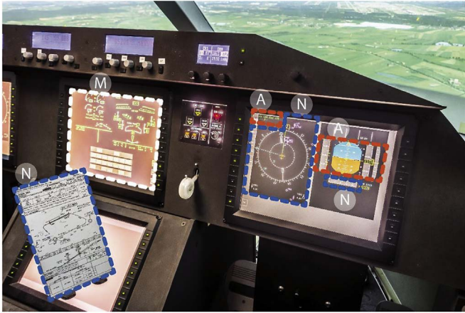
Fig. 2. Cockpit interior from participant's point of view showing the definition of Aol sets: Aviate (A), navigate (N), and system management (M).
