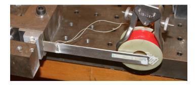
Figure 3: Experimental setup involving a cantilever beam controlled by two collocated piezoelectric patches.
