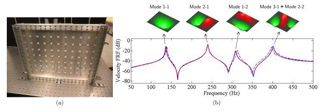
Figure 1: Experimental validation of the finite difference model: (a) Clamped plate. (b) Experimental operating deflection shapes with respect to the velocity FRF - (—) experimental FRF, (—) simulated FRF computed with  $15 \times 12$  unit cells.
