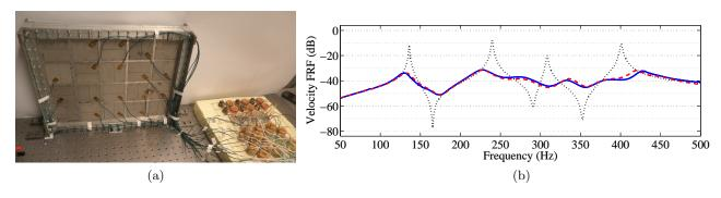
Figure 4: Coupling of the plate to its analogous network: (a) Clamped plate coupled to the electrical network through an array of  $5\times4$  piezoelectric patches. (b) Effect of the multimodal control on the velocity FRF of the plate -  $(\cdots)$  experimental FRF with short-circuited patches, (—) experimental FRF with the analogous network tuned to L=0.7 H and  $R_s=180~\Omega$ .
