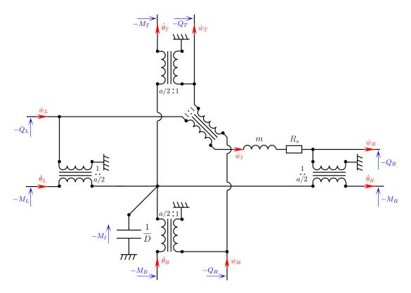
Figure 2: Electrical unit cell as a direct analogue of the finite difference model of a plate unit cell;  $R_s$  represents additional damping,  $R_s = 0$  when no damping is considered.
