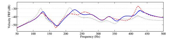
Figure 6: Influence of local defects - (—) optimal FRF with L = 0.7 H and  $R_s = 180 \Omega$ , (···) with a doubled mass in one mechanical unit cell, (—) with a doubled inductance in one electrical unit cell.
