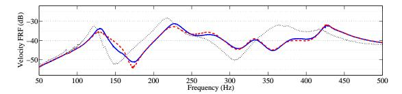
Figure 7: Influence of boundary conditions - (—) optimal FRF with L=0.7 H and  $R_s=180$   $\Omega$ , (···) with no bolts on the upper bar of the frame, (—) with the upper line of piezoelectric patches which is short-circuited.
