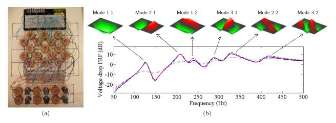
Figure 3: Experimental validation of the analogous network: (a) Electrical network implemented with  $5\times 4$  unit cells. (b) Experimental current distributions with respect to the voltage FRF with L=0.9 H and C=470 nF - (—) experimental FRF with  $R_s=0$   $\Omega$ , (--) simulated FRF with  $R_s=0$   $\Omega$ , (···) simulated FRF with  $R_s=180$   $\Omega$ .
