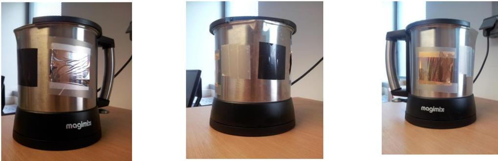
Measures of the respective emitted powers, indicated with equivalent temperature (IR “thermometer”/radiometer) when the water is boiling
