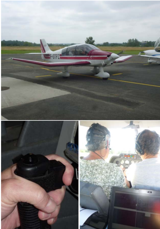
FIGURE 1 Experimental equipment and setup. Top: DR-400 Robin 4 seat airplane used in the experiment. Bottom left: Button response unit attached to the control stick. Used by the participant to identify when an audio alarm was heard. Bottom right: The configuration of individuals in the airplane consisted of the participant (pilot) in the front left seat (shown here wearing the Cognionics HD-72 dry-wireless 64 channel EEG system), the certified flight instructor in the front right seat, and the research engineer in the back right seat (experimental computer shown on research engineer's lap)
