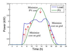
Figure 4. Optimal sizing method of PV system.
