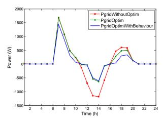
Figure 11. Grid power with and without management.
