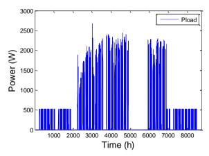
Figure 5. Building load profile in a typical year.
