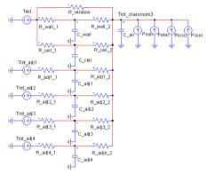
Figure 2. Equivalent electrical model of classroom 3.
