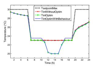
Figure 9. Controlled room temperature with and without optimal management.
