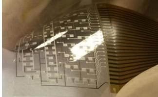
Fig. 7. Photograph of a 3-bit decoder with buffers.
