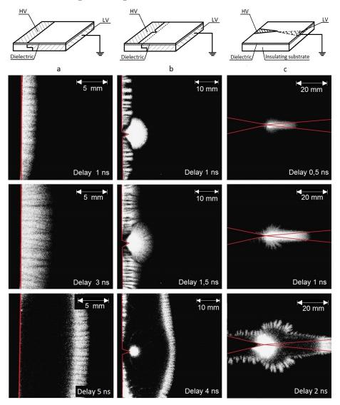
Figure 4. Evolution of SDBD in air for different geometries of the high voltage electrode in the system of flat electrodes. For all experiments the voltage of applied pulses was 30 kV on the electrode. ICCD camera gate is 1 ns.
