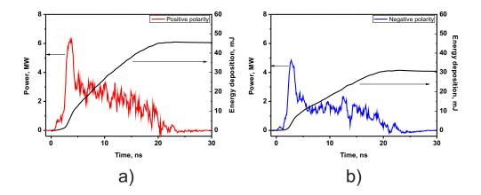
Figure 6. Power and energy deposited into the discharges for (a) positive and (b) negative polarities.
