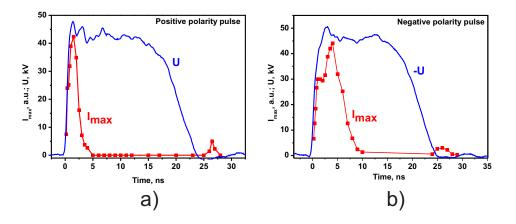
Figure 7. The peak intensities of the (0-0) line of 2+ system of molecular  $N_2$  for (a) positive and (b) negative polarities. Zone 0-1 mm form the high–voltage electrode.
