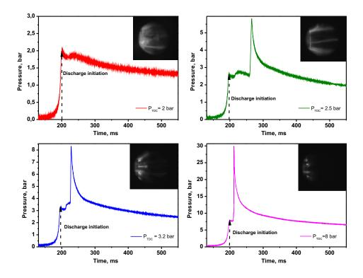
Figure 14. Pressure profiles in  $n-C_7H_{16}:O_2:N_2=1.8:19.6:78.6$  mixture at U = -46.9 kV and corresponding ICCD images of the discharge. ICCD gate is 100 ns.
