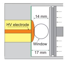
Figure 3. Optical access to the combustion chamber.
