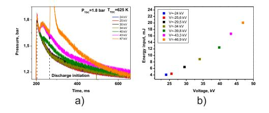
Figure 12. (a) Modification of pressure traces under the action of nanosecond surface dielectric barrier discharge,  $n-C_7H_{16}$ :  $N_2=1.8:19.6:78.6$  mixture,  $P_{TDC} = 1.8$  bar,  $T_C = 626$  K. Two nanosecond pulses, at time instance 210 ms and 270 ms, are applied to the system. Negative polarity pulses, voltage amplitude is between 24 and 46.9 kV. (b) deposited energy in the first pulse as a function of voltage amplitude on the high-voltage electrode in n-heptane-containing mixture.
