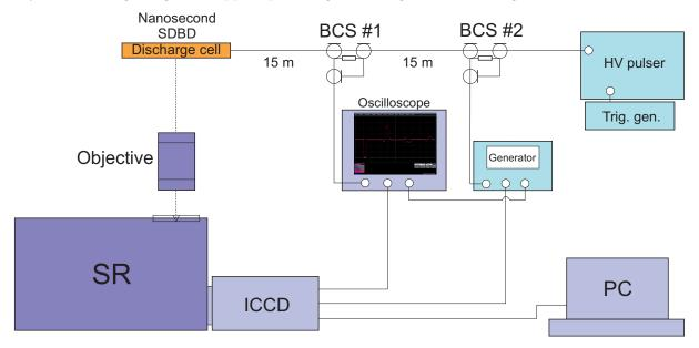
Figure 2. Scheme of experimental setup. BCS – back current shunt, SR – spectrometer, ICCD – ICCD camera, PC – computer.
