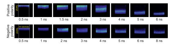
Figure 5. ICCD imaging of classical air flow electrode system. Gate of the camera is 0.5 ns.
