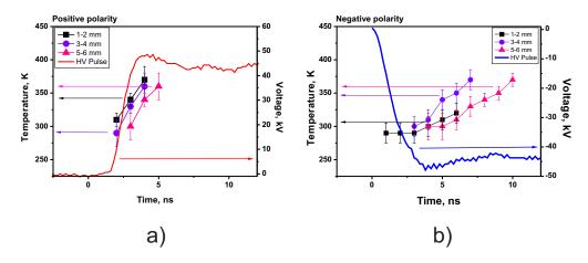
Figure 11. Time resolved rotational temperature for (a) positive and (b) negative polarity of applied pulses, taken at different distances from the high-voltage electrode.
