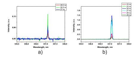
Figure 10. The spectra of line 337,1 nm on the trailing edge of (a) positive and (b) negative polarities of applied high-voltage pulses.
