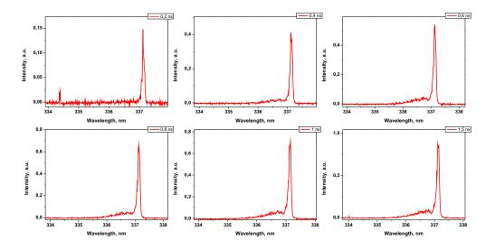
Figure 8. The spectra of line 337,1 nm on the leading edge. Positive polarity of high-voltage pulses.
