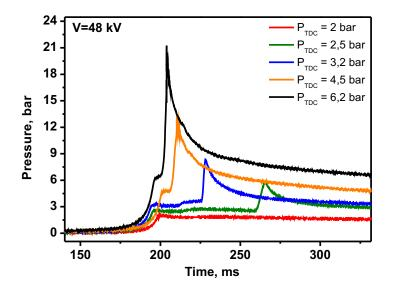
Figure 13. Modification of pressure traces under the action of nanosecond surface dielectric barrier discharge,  $n-C_7H_{16}:O_2:N_2=1.8:19.6:78.6$  mixture, different initial pressures. Negative polarity pulses, voltage amplitude is 46.9 kV.
