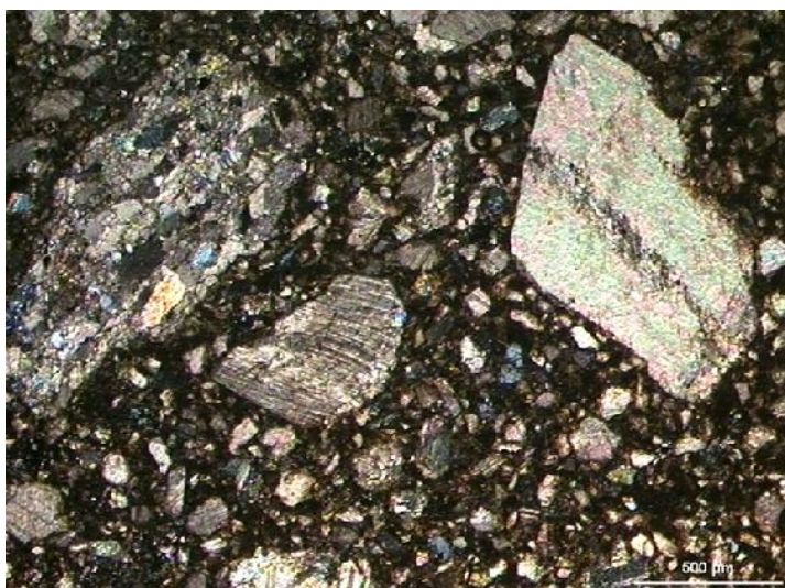
Fig. 4. The Fontana di Camerlata (render coat). White cement and aggregate of Musso marble (thin section)
