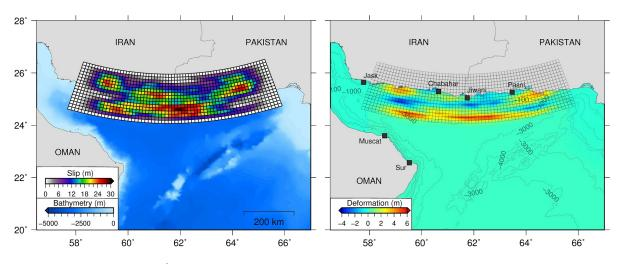
**Fig. 2.** An example of a  $k^{-2}$  slip model for the MAKRAN subduction zone (left panel) and the resulting vertical seafloor deformation (right panel). The non-planar mesh is the rupture geometry.
