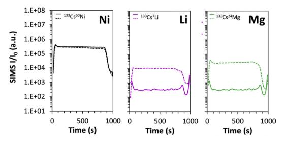
Fig. 1. SIMS depth profiling of elements Ni, Mg and Li in NiO (solid line) and NiO:(Li, Mg) 25 W (dashed line). Revised version.
