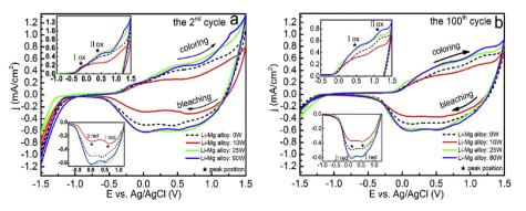
Fig. 7. (a) The 2nd and (b) 100th CVs of the NiO:(Li, Mg) films on ITO glass cycled in 1 M PC-LiClO<sub>4</sub> electrolyte with potential ±1.5 V for different Li-Mg powers. Ag/AgCl was used as reference electrode and Pt as counter electrode. Scan rate: 0.1 V/s, active area: 2.5 × 3 cm<sup>2</sup>.
