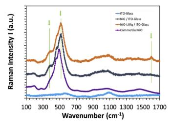
Fig. 4. Raman spectra of pure NiO and NiO:(Li, Mg) 25 W films with single ITO-glass and commercial NiO powder as reference.
