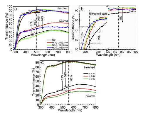
Fig. 11. (a) Transmittance curves, (b) partial enlargement for NiO:(Li, Mg) thin films at bleached and colored states with potential ±1.5 V and (c) for different potentials windows (±1.5 V, ±1.8 V, ±2.0 V) for NiO(Li, Mg) 25 W.
