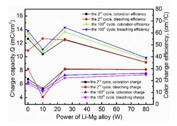
Fig. 9. Charge capacity and coloration efficiency of the NiO:(Li, Mg) films in 1 M LiClO<sub>4</sub>/ PC electrolyte.
