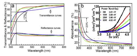
**Fig. 6.** (a) Transmittance and reflectance, (b) absorbance spectra of the NiO:(Li, Mg) thin films on quartz glass, Inset in panel (b) is plot of  $(\alpha hv)^2$  versus hv. (Black/red/green/blue curve corresponds to 0/10/25/80 W of Li-Mg power). (For interpretation of the references to color in this figure legend, the reader is referred to the Web version of this article.)
