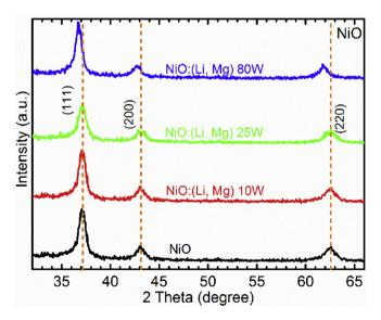
**Fig. 3.** XRD pattern for pure NiO (black line) and NiO:(Li, Mg) 10 W, 25 W and 80 W (red, green and blue curves) films. (For interpretation of the references to color in this figure legend, the reader is referred to the Web version of this article.)
