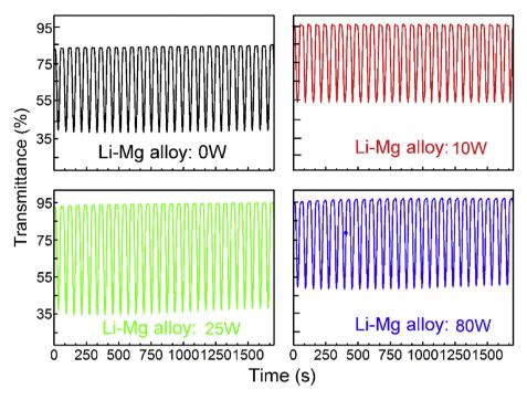
**Fig. 8.** *In situ* transmittance variation for the NiO:(Li, Mg) films at 550 nm cycled in 1 M PC– LiClO<sub>4</sub> electrolyte with potential ±1.5 V. Ag/AgCl was used as reference electrode and Pt as counter electrode. Scan rate: 0.1 V/s. (Black/red/green/blue curve corresponds to 0/10/25/80 W of Li-Mg power). (For interpretation of the references to color in this figure legend, the reader is referred to the Web version of this article.)
