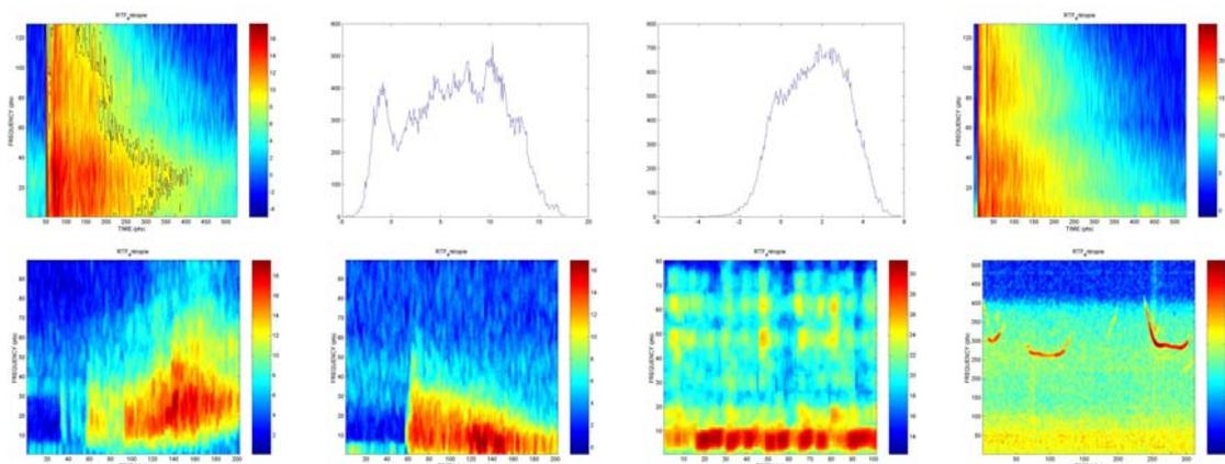
Figure 3: Entropy maps ( $\alpha=10$ ) for the signals of the figure 1. First line, entropy map of “Bastille” TFR, followed by its histogram and the RTF histogram, then the entropy map of “Halle aux grains”. Second line, entropy maps of avalanche, seismic, 1<sup>st</sup> type cavitation and bioacoustical signals.
