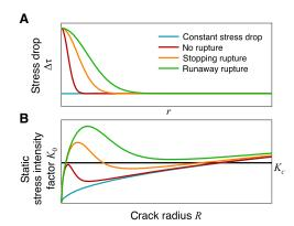
**Fig. 5. Fracture mechanics of rupture arrest under nonuniform stress.** Sketch of (**A**) stress drop distributions  $\Delta \tau(r)$  and (**B**) the corresponding static stress intensity factors  $K_0(R)$  illustrating different crack behavior (although our approach supports  $K_c$  being a function of R, for illustration purposes,  $K_c$  is plotted as a constant).
