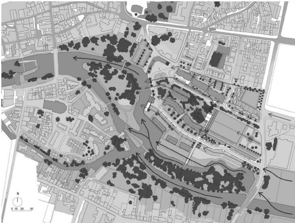
Figure 5. A neighbourhood designed as a temporary affluent of the river. The buildings are oriented parallel to the river and raised on stilts so as not to obstruct the flow of water in the event of flooding. Source: EDL architect
