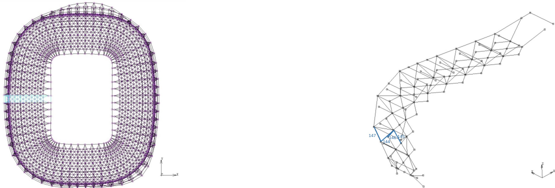
Fig. 2 Finite element model of the roof structure (left) and zoom (right) in the structural zone corresponding to the light color part shown in the left figure (from CSTB).
