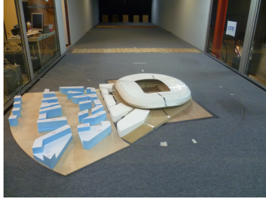
Fig. 1 Model of the roof of the Allianz Riviera stadium in the boundary layer wind tunnel at CSTB in Nantes (Vinet and De Oliveira 2013).
