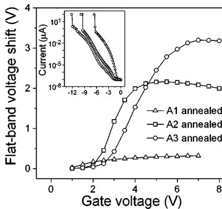
FIG. 4. Flat-band voltage shift ( $\Delta V_{FB}$ ) as a function of the gate voltage round sweep for 7-nm-thick oxide layers implanted with  $2 \times 10^{16}$  Si/cm<sup>2</sup> at 1 keV and subsequently annealed following the A1, A2, or A3 treatment. Inset: Magnitude of the dark gate current under accumulation conditions as a function of negative ramped gate voltage (1 V/s).
