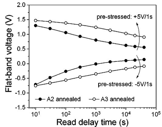
FIG. 5. Data retention characteristics of 7-nm-thick oxide layers implanted with  $2 \times 10^{16}$  Si/cm<sup>2</sup> at 1 keV and subsequently A2 or A3 annealed. The magnitude of the applied gate voltage stress was +5 V or -5 V for 1 s.
