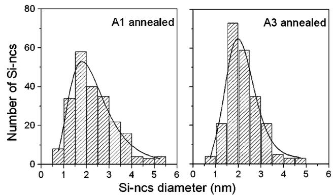
FIG. 2. Nanocrystal size distribution measured from plane-view TEM images of 7-nm-thick SiO<sub>2</sub> annealed according to the A1 or A3 treatment. The number-average size (mean size) is around of 2 nm for both samples.
