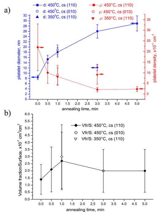
**FIGURE 5.** Evolution of a) mean platelet diameter and surface density and b) platelet volume fraction per square unit as a function of annealing condition.
