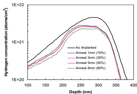
**FIGURE 2.** Comparison of SIMS profiles from Si implanted with H-ions, before and after isothermal anneals at 450°C.
