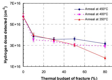
**FIGURE 3.** Time-evolution of hydrogen dose measured by SIMS after isothermal anneals at 350, 400 and 450°C as a function of the thermal budget of fracture.
