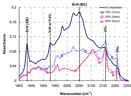
**FIGURE 4.** FTIR spectra of the Si-H stretching modes of H implanted Si, before and after isothermal anneals at 450°C.
