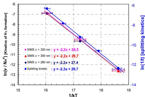
**FIGURE 6.** Comparison between the splitting kinetics reference and the calculated kinetics of H<sub>2</sub> formation (i.e. decrease of H-measured by SIMS) during the entire thermal treatments.
