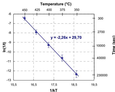
**FIGURE 1.** Splitting kinetics of Si implanted with an energy in the range of 40 keV and a few  $10^{16}$   $H^+$ /cm $^2$ .
