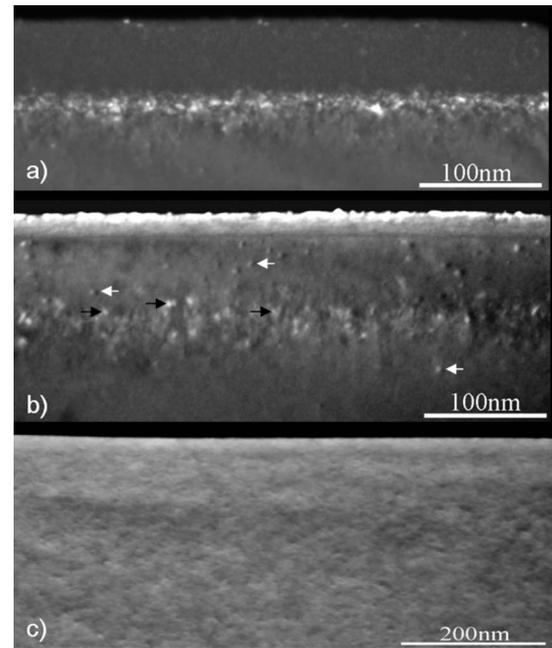
FIG. 1. A series of cross-section TEM images showing (a) the as-implanted area, (b) the laser spot area irradiated with energy fluence of 3 mJ/mm<sup>2</sup>, and (c) the laser spot area after irradiated with energy fluence of 4 mJ/mm<sup>2</sup>.
