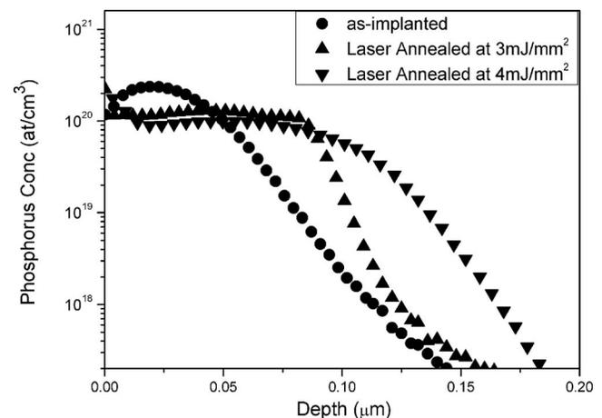
FIG. 2. SIMS measurements showing phosphorus depth profiles for the as-implanted sample and for the samples irradiated with energy fluences of 3 and 4 mJ/mm<sup>2</sup>. In order to increase clarity data points shown in the graph are reduced.
