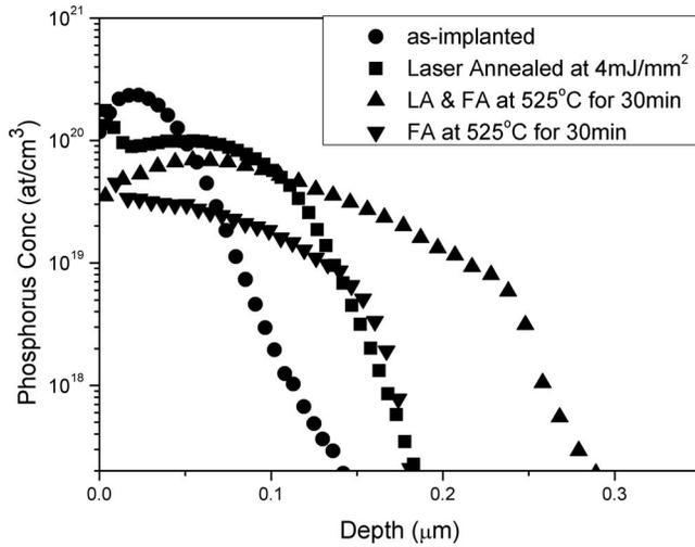
FIG. 3. Phosphorus depth profiles obtained by SIMS measurements showing the effect of conventional furnace annealing at temperature of 525 °C for 30 min both at LA (4 mJ/mm<sup>2</sup>) and as-implanted areas. Depicted data points are reduced.
