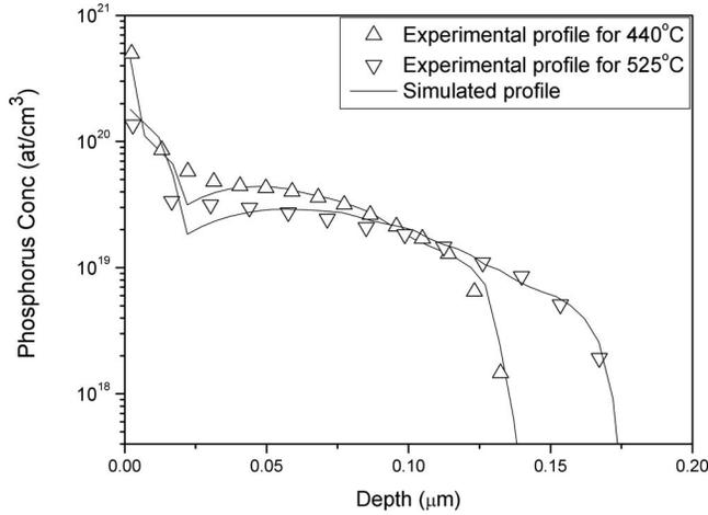
FIG. 5. SIMS depth profile after furnace annealing at 440 °C (opened triangle up  $\Delta$ ) and 525 °C (opened triangle down  $\nabla$ ) for 30 min against the best fit simulated profiles obtained by doubly charged diffusivity model (solid line) considering a maximum electrical activation of  $1.0 \times 10^{19} \text{ cm}^{-2}$ . Data points are reduced.
