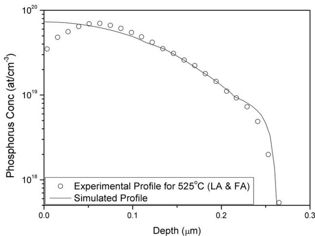
FIG. 6. Phosphorus depth profile obtained by SIMS measurement after conventional furnace annealing at temperature of 525 °C for 30 min at LA ( $4 \text{ mJ/mm}^2$ ) area against the best fit simulated profile obtained by doubly charged diffusivity model (solid line) considering a maximum electrical activation of  $1.0 \times 10^{19} \text{ cm}^{-2}$ . Depicted data points are reduced for clarity.
