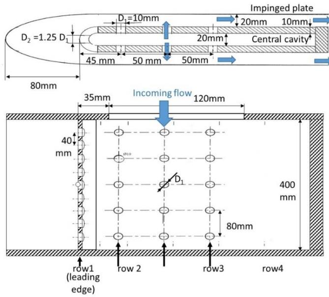
Figure 2. Test section
