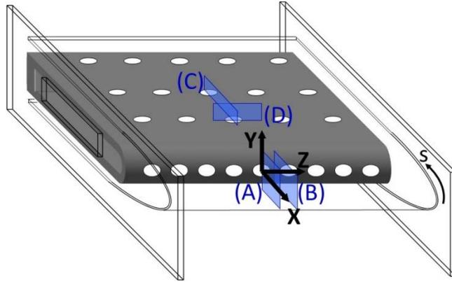
Figure 3. PIV measurements planes
