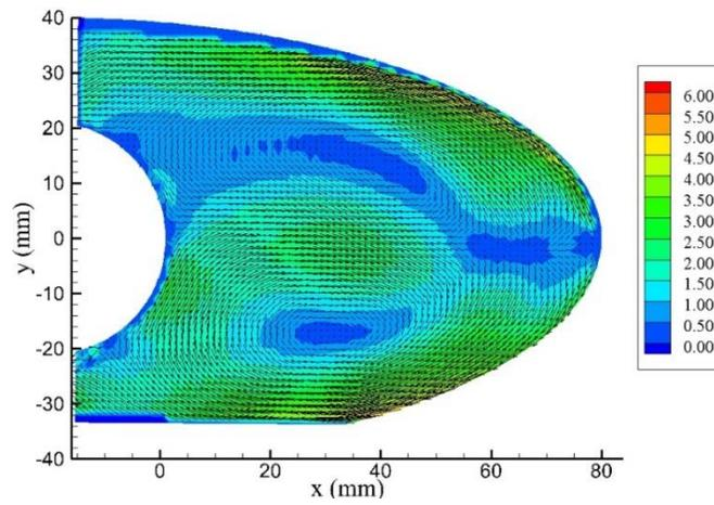
Figure 15 . Velocity Magnitude Distribution , plane (B), PIV
