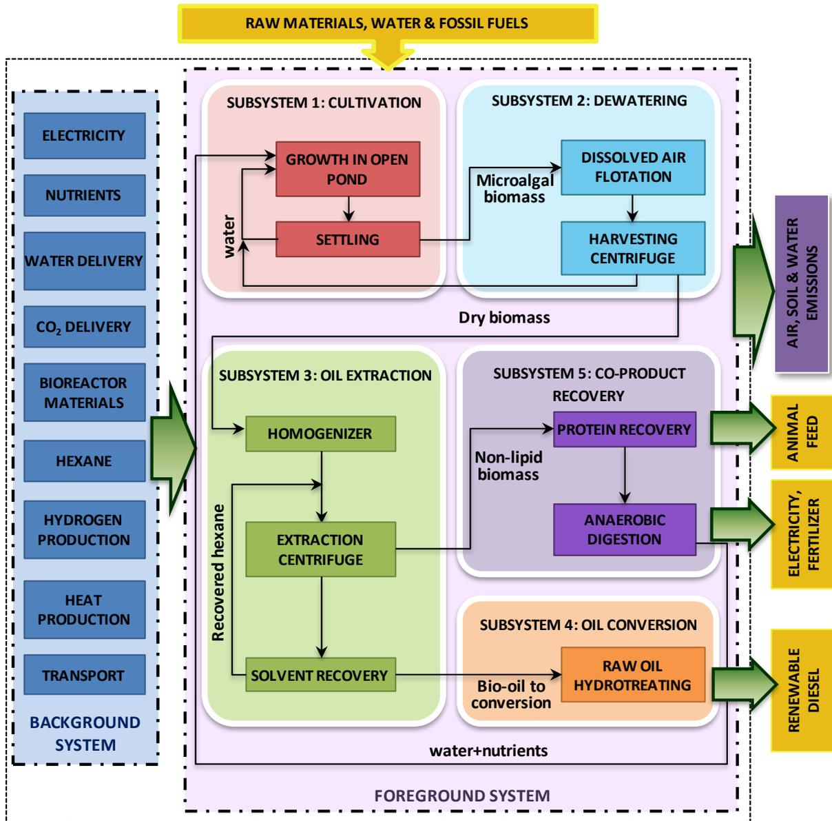
**Figure 1.** Process chain and system boundaries of the microalgal biorefinery for the simultaneous production of renewable diesel, animal feed and fertilizer fraction coupled to energy recovery by AD.
