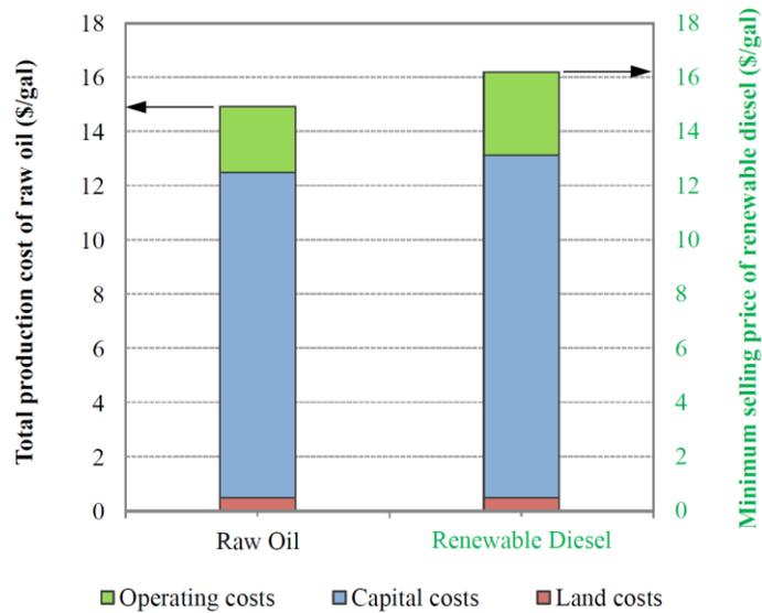
**Figure 2.** Environmental and economic results for harmonized scenario: a) Relative contributions of microalgal production of renewable diesel, protein fraction and fertilizer coupled to energy recovery by AD per stage and b) Breakdown of oil production costs (blue axis) and diesel minimum selling price (red axis), considering 10% MARR and 2011 as the base year.
