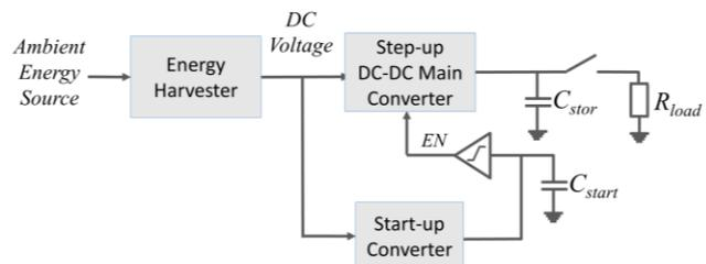
Fig. 1: Overall architecture of the conversion circuit
