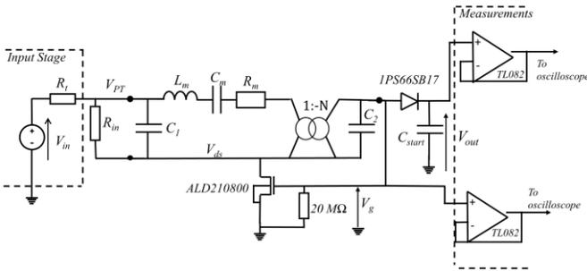
Fig. 11: Circuit of the experimental test bench
