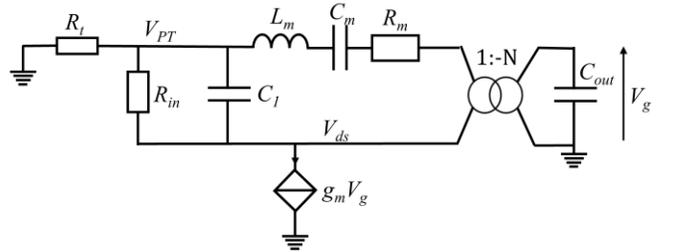
Fig. 5: Small-signal equivalent circuit
