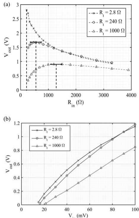
Fig. 16: Output voltage gain for different harvester resistances (a) as a function of  $R_{in}$  and for  $V_{in} = 100$  mV and (b) as a function of  $V_{in}$  for a biasing resistance  $R_{in} = 2200 \Omega$
