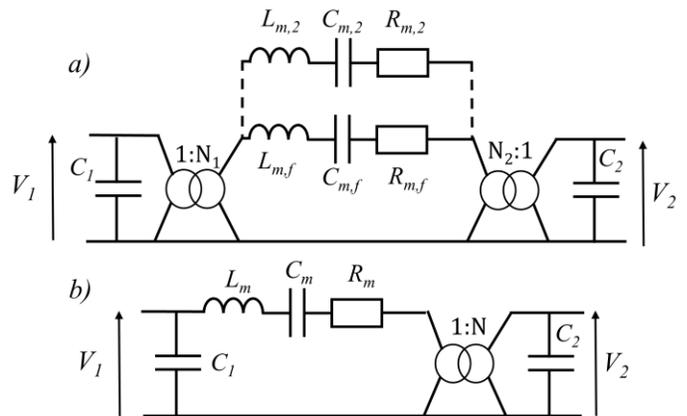
Fig. 2 (a) Equivalent circuit of a PT
