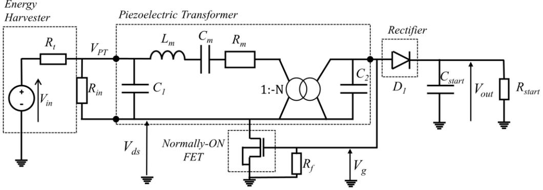
Fig. 4: Circuit Schematic
