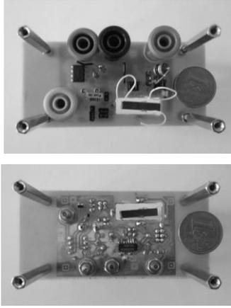
Fig. 10: PCB of the proposed start-up converter.
