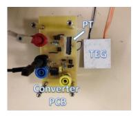
**Figure 4.** PCB of the proposed start-up converter.
