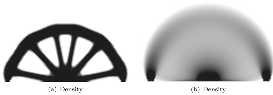
Figure 9: Optimized design of the bridge with penalized (a) and non penalized (b) SIMP method
