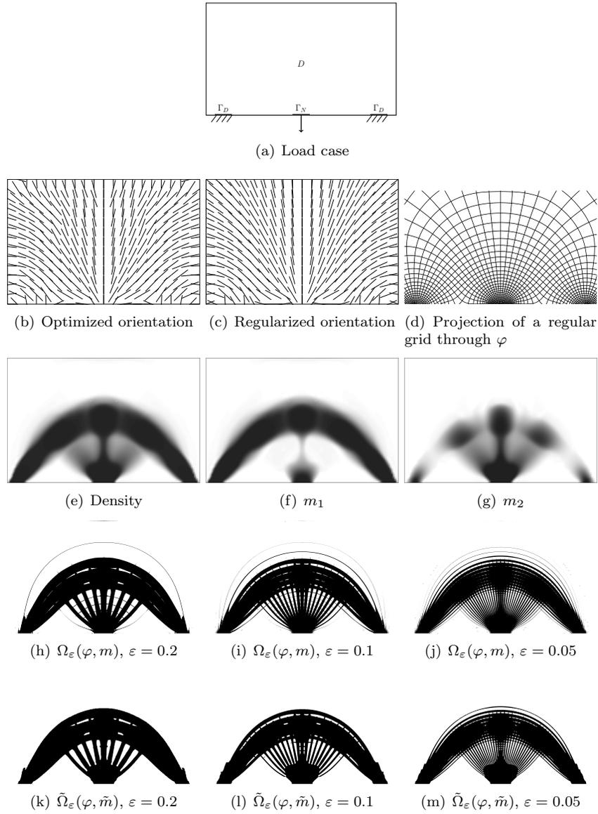
Figure 25: Complete process for an arch case
