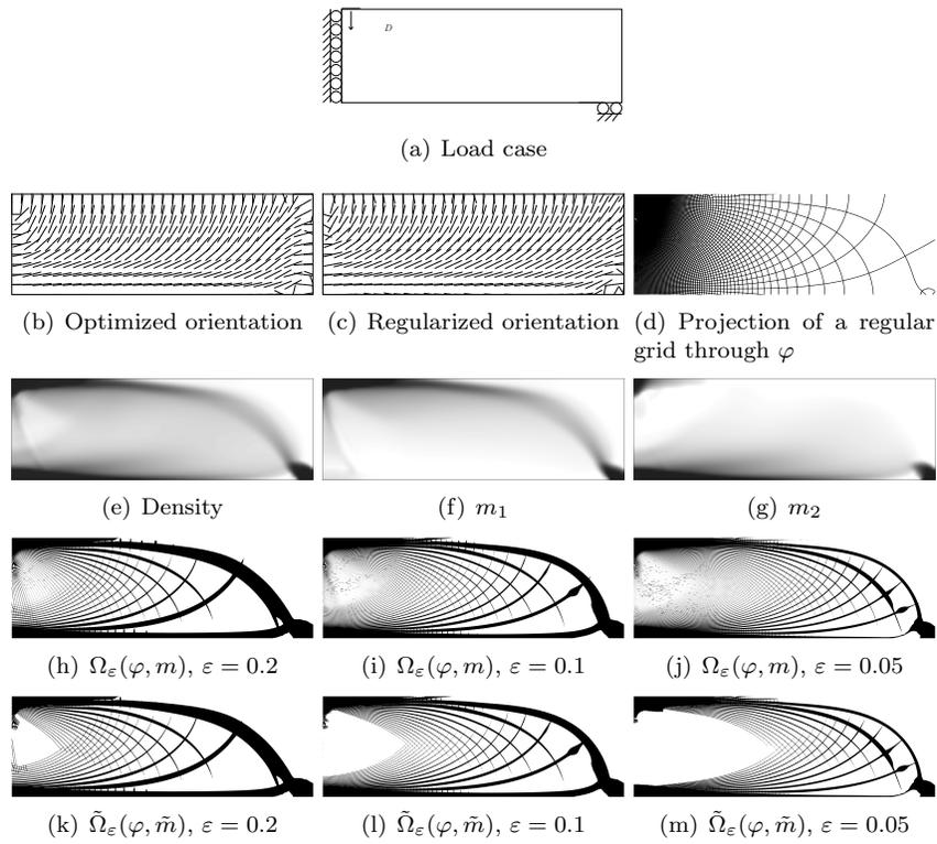
Figure 27: Complete process for a MBB beam
