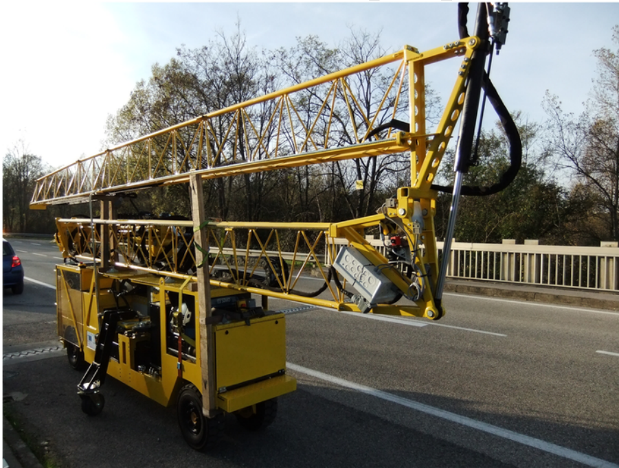
Fig. 6. Mobile robot in approach stage for a road bridge inspection. The cabin and the arm are folded. The lateral stabilizing wheels are deployed.
