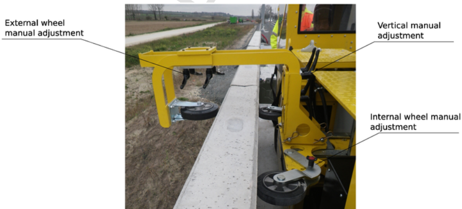
Fig. 9. Parapet slider installed on a parapet.
