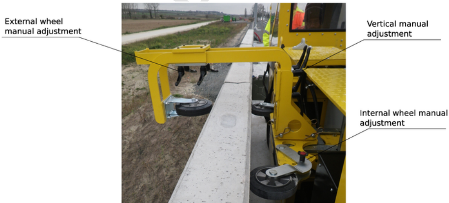
Fig. 9. Parapet slider installed on a parapet.
