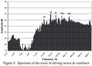
measured with 3555 rpm (1/12 octave)
