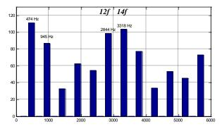
Figure 5. Total analytical vibratory spectrum with 3555 rpm.
