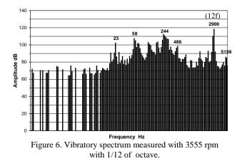
In order to study the vibrations generated by the operating conditions, an accelerometer is positioned on the frame of the machine. It measures the deformations of the frame. The vibratory spectrum gives lines identical to those obtained by the noise measurement; it displays a dominant line situated at 2900 Hz, that corresponds to the theoretical excitation mode 0 predicted at 2844 Hz (Figure 6).
