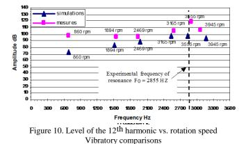
To know which lines to reduce does not require to know its amplitude precisely. Its frequency, on the other hand, must be well given. Lastly, taking into account the complexity of the studied phenomena and the many steps of calculations making it possible to lead to the results, the latter seem very satisfactory.
