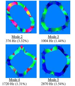
Figure 4. Mode shape, resonance frequencies with (<u>damping</u> <u>coef.</u>) obtained by measurements
