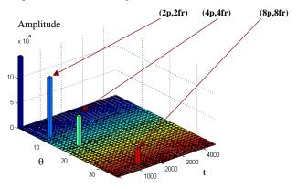
Figure 3. FFT 2D of radial force ( $fr = p \times N$ )
