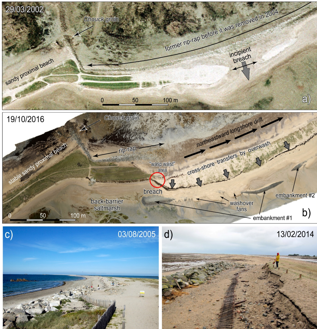
Fig. 9. Morphological changes of the proximal section situated on both sides of the Chouck groin over the whole survey period: (a) 29/03/2002 (source: IGN - CA00S01232_FR5415_250_1181); (b) 19/10/2016. Shoreline retreat of the gravel proximal section between 2005 (c) and 2014 (d). This section called “wasp waist” is nowadays threatening to break.
