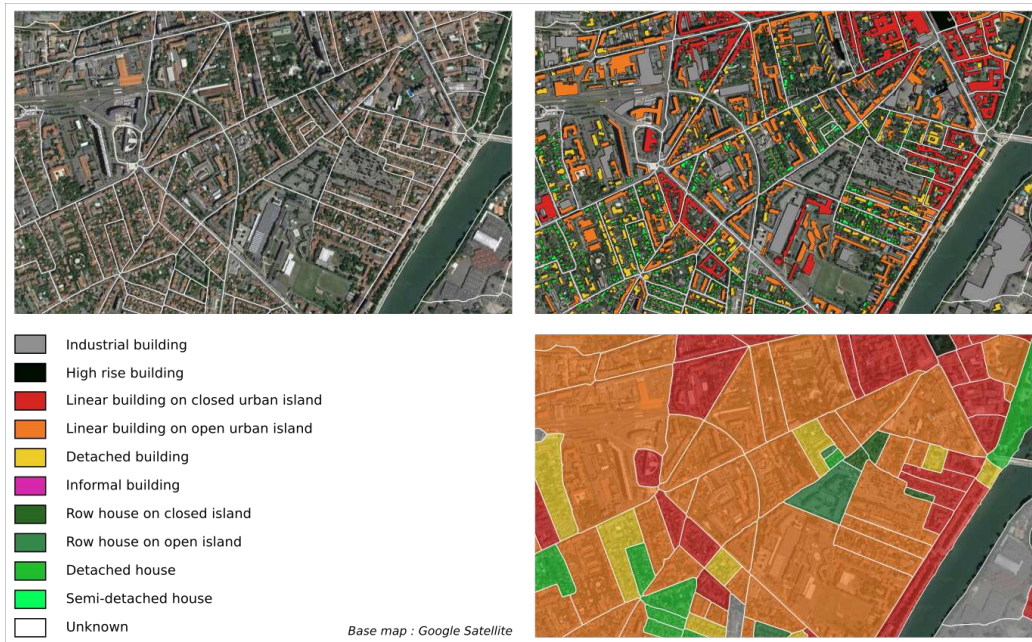
Figure 9: Comparison between the satellite image (top left) and the urban fabric typology classification at the building level (top right) and RSU level (bottom right) in the French municipality of Toulouse
