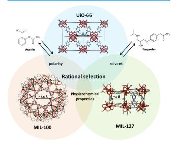
**Figure 1.** Schematic view of the structure of UiO-66, MIL-100, and MIL-127 (zirconium polyhedra, iron polyhedra, nitrogen, oxygen, and carbon are represented in cyan, green, blue, red, and gray, respectively; hydrogen atoms are omitted for clarity). Structures of AAS and IBU drugs are also given.
