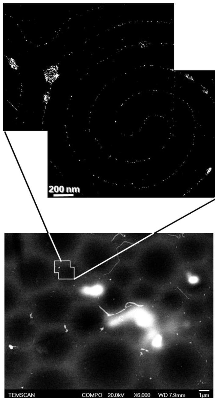
**Fig. 5.** Magnified view of a double spiral for film as thin as possible—close to 2 μm (SEM, backscattered electrons mode). This situation corresponds to a spiral with a very thin arm made with a significantly reduced number of gold nanoparticles.
