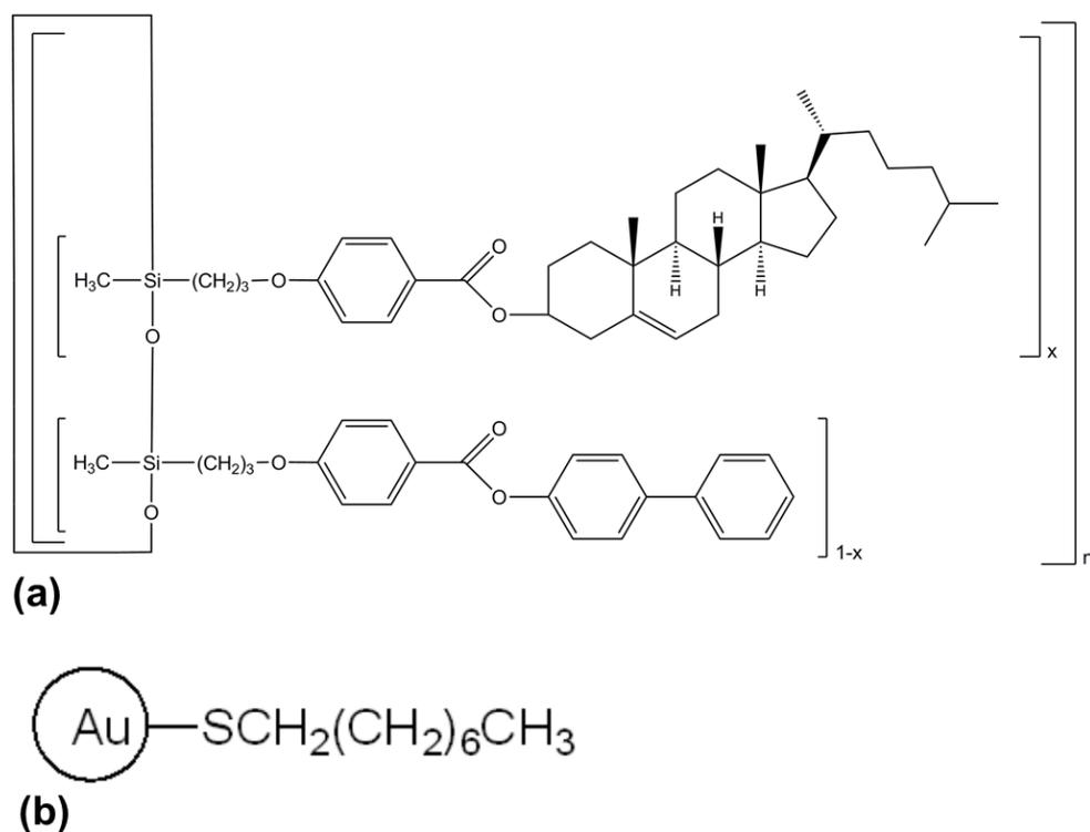
**Fig. 1.** Chemical structure of materials. (a) Cholesteric liquid crystal oligomers (image courtesy of Dr. E. Hanelt). The quantity  $x$  is the molar fraction of the chiral mesogen and  $n$  represents the ring size of the siloxane backbone. (b) Gold nanoparticle functionalized with octanethiol.
