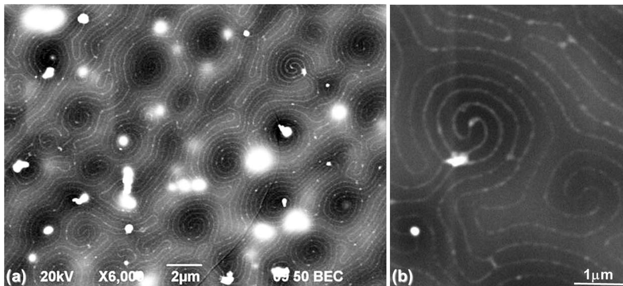
**Fig. 3.** (a) Network of double spiral cholesteric patterns of gold nanoparticles. (b) Magnified view of a pair of double spirals. SEM (backscattered electron mode). Gold appears everywhere in white and light grey. Film thickness was 13  $\mu\text{m}$ .
