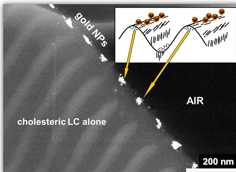
**Fig. 7.** Cross-sectional view of cholesteric film doped with gold nanoparticles showing the correspondence between fingerprint texture of a pure liquid crystal and localization of nanoparticles at the free surface of the film after annealing (18 h). HAADF-STEM. Insert: scheme to show the relation between the position of nanoparticles at the free surface and the orientation of rod-like liquid crystalline molecules at the immediate surrounding.
