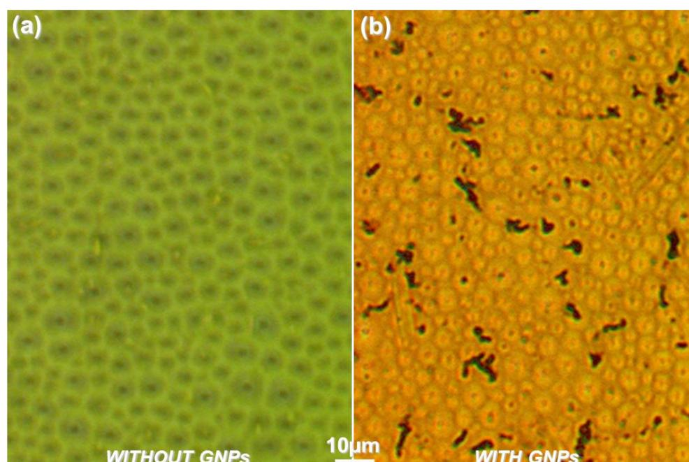
**Fig. 2.** Optical textures of cholesteric films (a) without and (b) with gold nanoparticles. Film thickness was 13  $\mu\text{m}$ . Data acquired in transmission mode and incident light was unpolarized.
