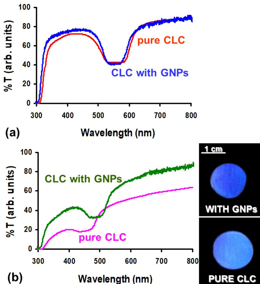
**Fig. 9.** Transmittance spectra of cholesteric films with and without gold nanoparticles (a) before and (b) after annealing (18 h). Inset shows images of experimental cells after annealing with and without gold nanoparticles. Film thickness was 13  $\mu\text{m}$ .
