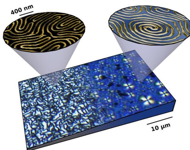
*Gold nanoparticles are patterned on demand into various cholesteric textures by playing with the film thickness and the interfacial properties*
