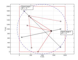
Fig. 1. Target trajectories. A circle " $\bigcirc$ " indicates where a trajectory begins, and a square " $\square$ " indicates where a trajectory ends. The large square indicates the limits of the sensor's field of view (FoV) and the large dashed circle represents the 90% confidence region of the Gaussian component of the spontaneous birth model
