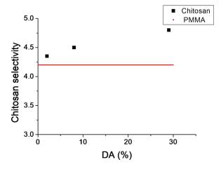
Fig. 5. (Color online) Selectivity of chitosan compared to PMMA for 2%, 8% and 35% DA for CHF<sub>3</sub> plasma. Dashed line corresponds to PMMA selectivity. Chitosan and PMMA were filmed on 200 nm thick PECVD-deposited SiO<sub>2</sub>. Chitosan (or PMMA) selectivity corresponds to the ratio of SiO<sub>2</sub> etching rate on chitosan (or PMMA) etching rate.
