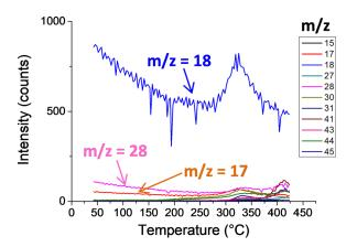
Fig. 3. (Color online) TPD-MS spectrum of a film of chitosan of DA 2% after spin-coating and after a softbake at  $100\,^{\circ}$ C during 1 min. Each curve represents a ratio m/z.
