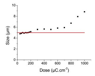
Fig. 7. (Color online) Effect of the dose on the size of a pattern of  $5 \mu m$ . Red line corresponds to the aim of  $5 \mu m$  in size.
