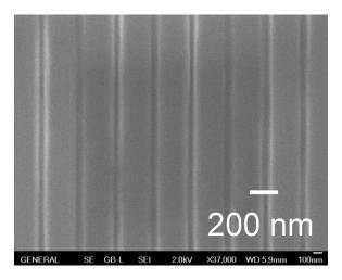
Fig. 9. SEM image of patterns obtained by EB lithography at  $180 \,\mu\text{C cm}^{-2}$  on chitosan after transfer by CHF<sub>3</sub> plasma etching and stripping of chitosan 47 nm line and 332 nm space on the average of 50 measures.
