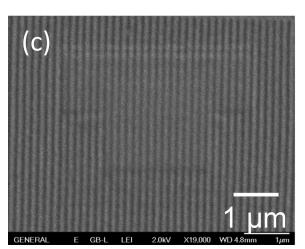
Fig. 8. SEM images of nanopatterns obtained by EB lithography at  $30 \,\mathrm{kV}$  and  $10 \,\mathrm{pA}$  in a chitosan positive resist at an optimal dose range between  $180 \,\mathrm{and} \,220 \,\mu\mathrm{C} \,\mathrm{cm}^{-2}$ . Average feature sizes on 50 measures are (a) 65 nm line and  $505 \,\mathrm{nm}$  space, (b)  $70 \,\mathrm{nm}$  line and  $288 \,\mathrm{nm}$  space, and (c)  $59 \,\mathrm{nm}$  line and  $97 \,\mathrm{nm}$  space.
