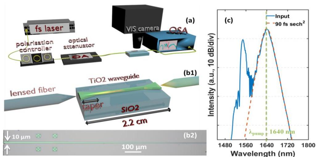
**Figure 2:** (a) Experimental setup involved for generation of supercontinuum in  $\text{TiO}_2$  waveguides. (b1) sketch of the waveguide with the coupling by lensed fiber and (b2) the corresponding optical microscope image of the taper used for the coupling. (c) Spectrum of the input soliton pulse centered at  $1640 \text{ nm}$  compared with the spectrum of a  $90 \text{ fs sech}^2$  pulse (c)
