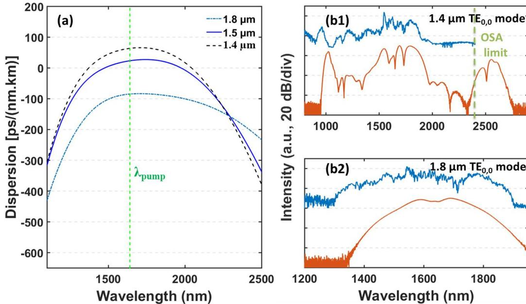
**Figure 6:** (a) Dispersion profiles of the fundamental TE<sub>0,0</sub> mode of the waveguide for different widths (1.4, 1.5 and 1.8  $\mu\text{m}$ ). (b) Experimental spectra (blue lines) and corresponding numerical simulations (red lines) for (b1) 1.4  $\mu\text{m}$  and (b2) 1.8  $\mu\text{m}$ . For the clarity of the figure, the various spectra were vertically offset.
