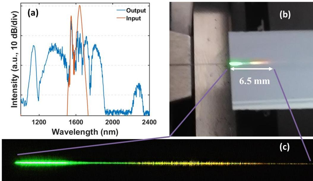
**Figure 3:** (a) Optical supercontinuum recorded at the output of the 2.2-cm-long 1.5- $\mu\text{m}$ -wide  $\text{TiO}_2$  waveguide (blue solid line) compared to the input pulse spectrum (red solid line). The overall spectrum is reconstructed from the overlap of the spectra obtained from both optical spectrum analyzers of our setup. (b) Photography of the visible light emitted from the waveguide. (c) Zoom of the emitted visible light.
