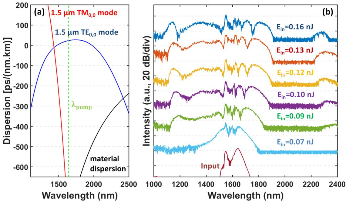
**Figure 4:** (a) Dispersion profiles of the fundamental TE<sub>0,0</sub> and TM<sub>0,0</sub> modes of the 1.5  $\mu\text{m}$  wide waveguide. The material dispersion is plotted with solid black line. (b) Optical supercontinua measured at the output of the TiO<sub>2</sub> waveguide for various coupled energy conditions. For the better reading of the figure, the various spectra were vertically offset.
