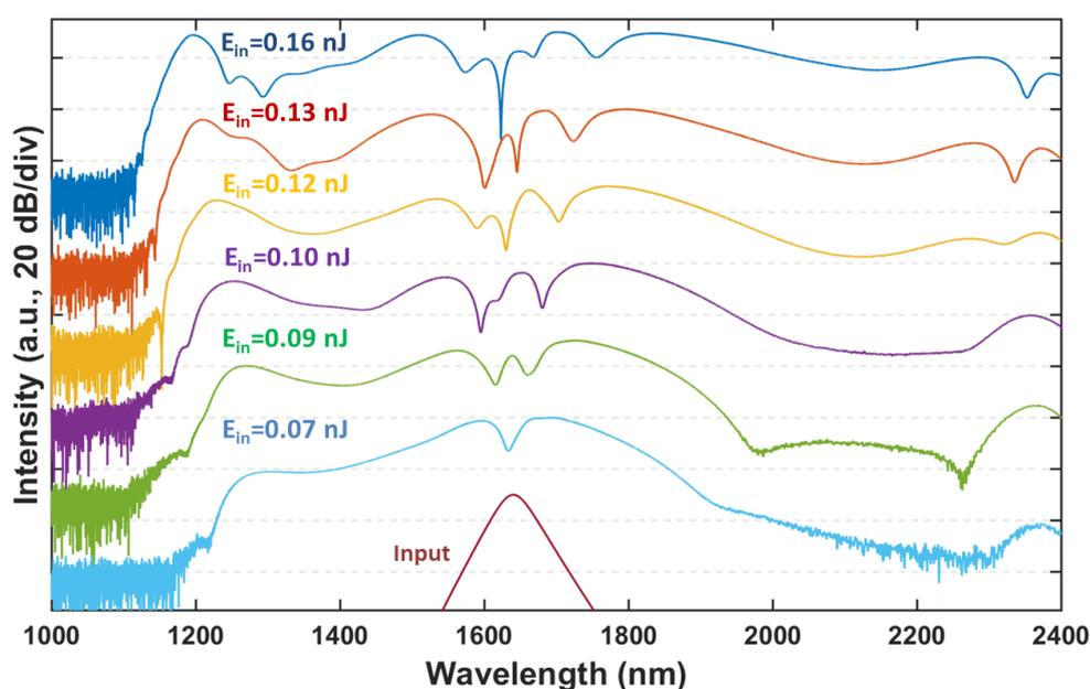
**Figure 5:** Numerical simulations of supercontinuum generation obtained in a 2.2-cm-long 1.5- $\mu\text{m}$ -wide TiO<sub>2</sub> waveguides for different input energies of the femtosecond pulses. For the clarity of the figure, the various spectra were vertically offset.
