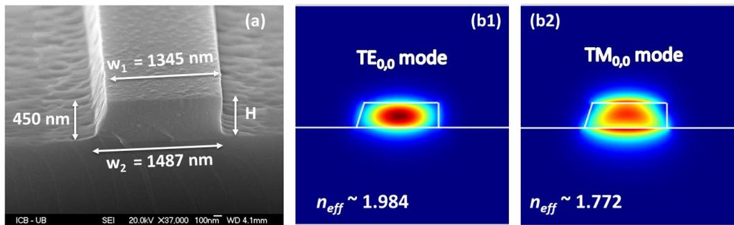
**Figure 1:** (a) Scanning Electron Microscope image of the cleaved strip TiO<sub>2</sub> waveguide (b1 & b2) Corresponding mode profiles at 1640 nm and associated effective index for the first transverse electric (TE) and transverse magnetic (TM) respectively.
