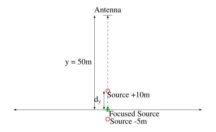
Figure 9: Configuration used to simulate the position error in distance
