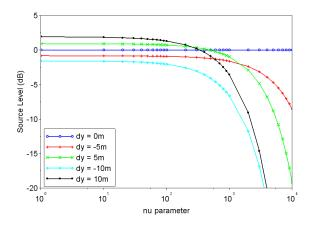
Figure 10: Source level as a function of the parameter v for different distance errors
