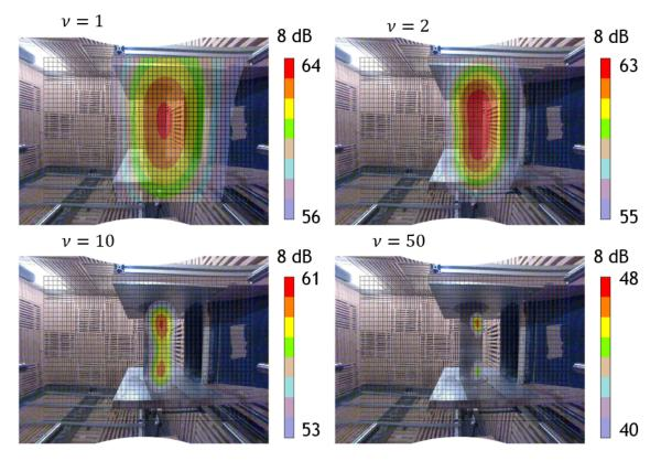
*Figure 15: FBF localization results for the aeroacoustic case at* 1kHz (v = 1, 2, 10, 50)
