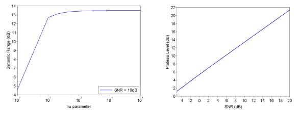
(a) Dynamic obtained as a function of v for a source(b) Plateau level in function of the injected noise and an uncorrelated noise (SNR = 10dB) power
