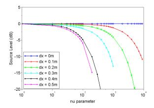
Figure 7: Source level as a function of the parameter v for grid errors.  $d_x = 0 m$ : source on a grid point,  $d_x = 0.5 m$ : source midway between two grid points
