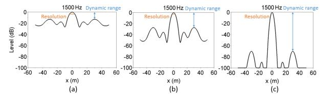
Figure 2: FBF on a single source (x = 0 m) in a 1D case for a: v = 1 (CBF), b: v = 2 and c: v = 5
