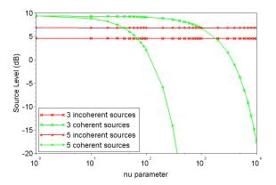
Figure 11: Source level in function of the parameter v for coherent and incoherent sources
