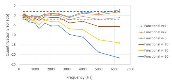
*Figure 13: Gap between source level with FBF and the intensimetry reference (for* v = 1, 2, 5, 10, 20, 30)
