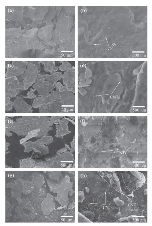
Fig. 4. FESEM images of the MWCNT/Al powders (a-b) P0.5, (c-d) P1, (e-f) P1.5 and (g-h) P2.
