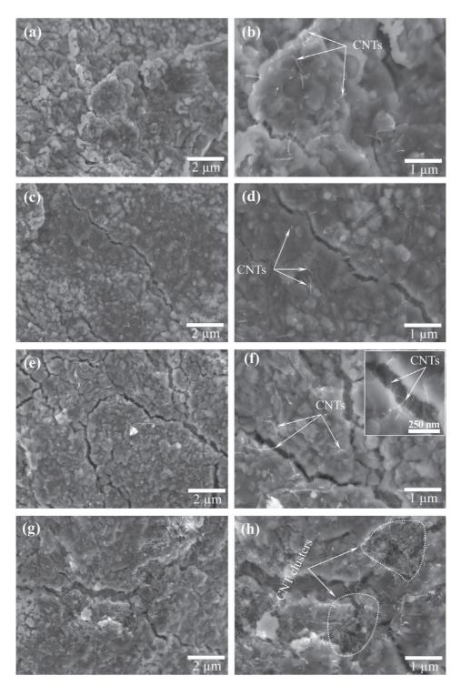
Fig. 11. Top-view FESEM images in Area 1 for (a-b) S 0.5, (c-d) S1, (e-f) S1.5 and (g-h) S2. Inset in (f) shows crack bridging by the MWCNTs.
