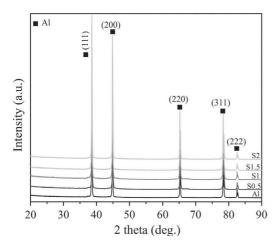
Fig. 6. XRD patterns of sintered specimen S0 (Al), S0.5, S1, S1.5 and S2.
