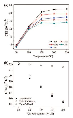
**Fig. 13.** (a) CTE of CNT/Al composites versus temperature and (b) comparison between calculated and experimental CTE versus carbon content in the temperature range of 200–250 °C. (For interpretation of the references to color in this figure legend, the reader is referred to the web version of this article.)
