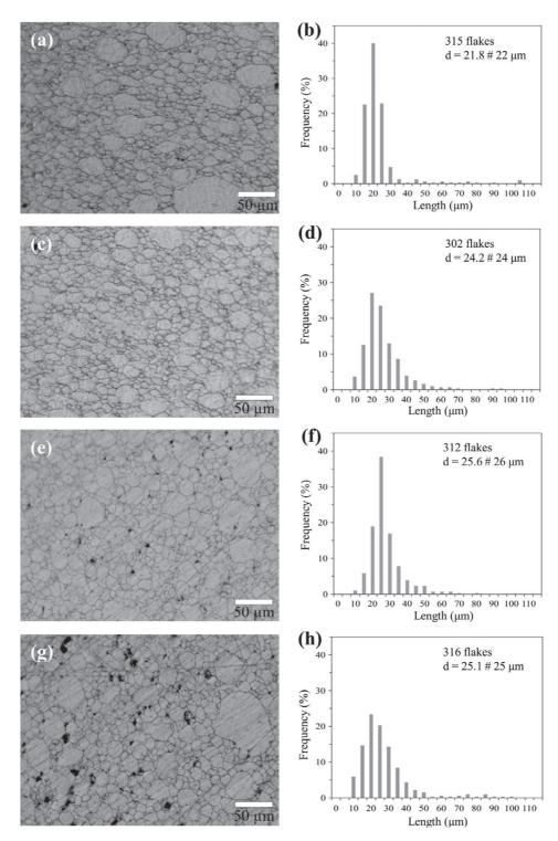
Fig. 8. Top-view optical images and flake size distribution of the sintered specimens (a-b) S0, (c-d) S0.5, (e-f) S1.5 and (g-h) S2.
