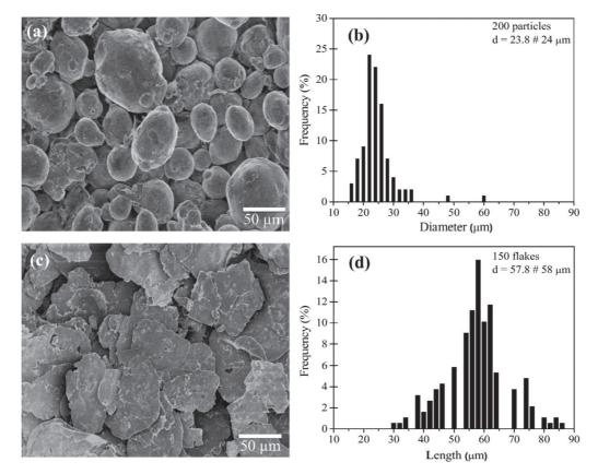
Fig. 1. FESEM images and grain size distributions of (a, b) the as-received Al powder and (c, d) after ball-milling resulting in Al flakes formation.
