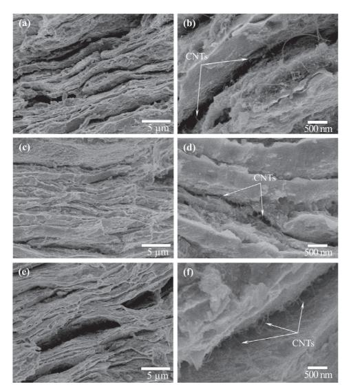
Fig. 12. Cross-section FESEM images of S1 at different positions (e) from center to periphery (a-b) Area 1 (c-d), Area 2 and (e-f) Area 3.
