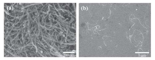
Fig. 2. FESEM images of MWCNTs (a) as-received and (b) dispersed in water then dropletted on a Si substrate.
