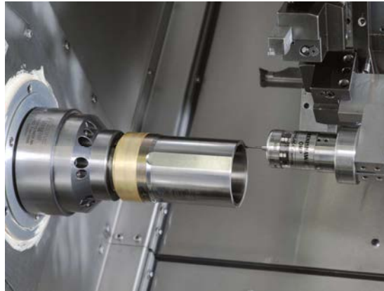
Fig. 5: PtRh10 test-mass mounted at a brass adapter and testing probe inside the precision fabrication station
