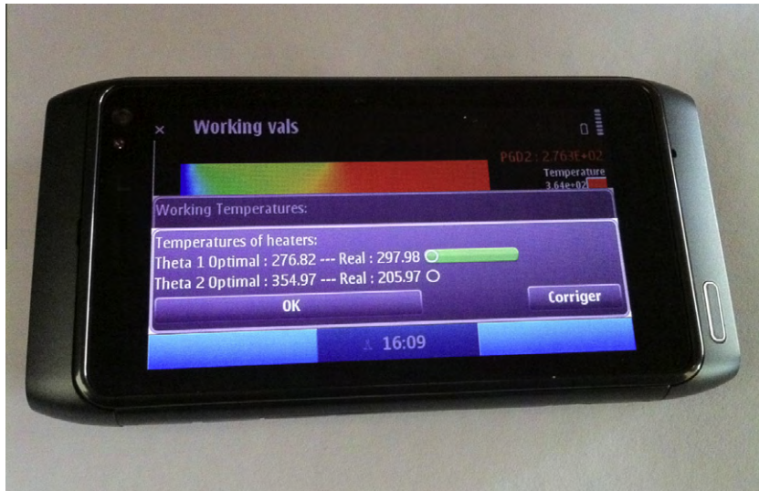
Fig. 11. Identification of the real process parameters, i.e. the real temperatures of both heating devices.
