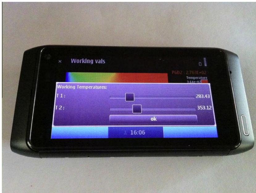
Fig. 8. Optimal temperatures at positions P_1 and P_2 when both heaters work at the optimal conditions.
