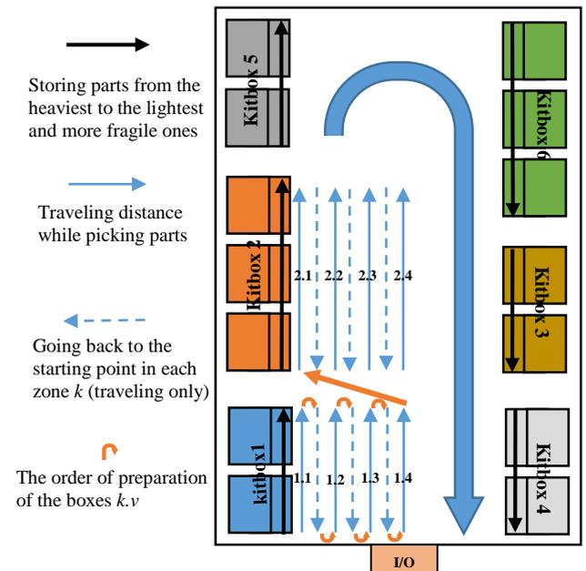
Figure 4: Representation the robot's traveling to prepare boxes  $k.v$
