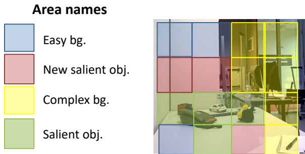
Fig. 19. The 16 regions are classified according to 4 groups (of a different color). Recall that these regions were defined by dividing the pan-tilt space into 16 equally-spaced squares. Their approximative positions are projected on this image as an example.
