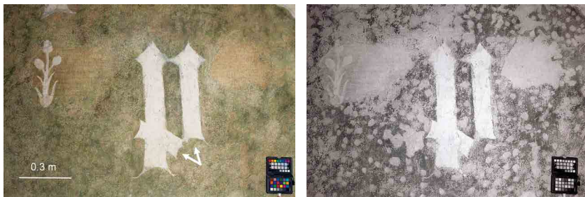
Figure 4.4. VIS and IR (approx. 830–1000 nm) photographic images of the letter P highlighted in figure 4.3. Arabesques in the lower part of the letter P are indicated in the VIS image. They seem to disappear in the IR image. Photos: Francesca Piqué, 2016.
