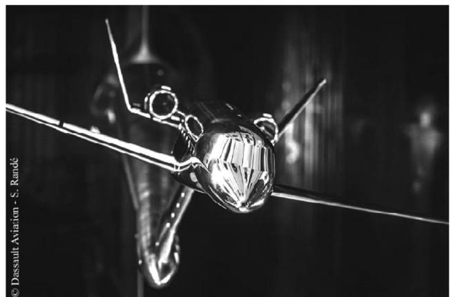
Fig. 1 LSBJ model in ETW test section.
