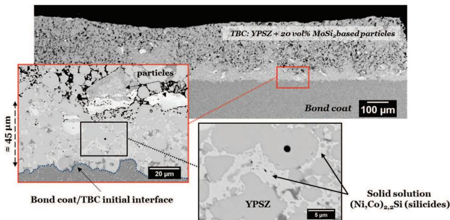
Fig. 5. SEM backscatter electron image of a cross-section of a TBC system as manufactured by spark plasma sintering highlighting the occurrence of a reaction between the MoSi<sub>2</sub> based particles and the NiCoCrAlY bond coating leading to the formation of (Ni, Co)<sub>2,2</sub>Si silicide.
