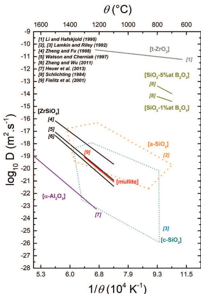
Fig. 4. Diffusion coefficient of oxygen D as a function of temperature  $\theta$  for zirconia [41], silica [42], mullite [43], alumina [44] and zircon [45–47]. Domains for oxygen diffusion in amorphous and crystalline silica are reproduced from Ref. [48].
