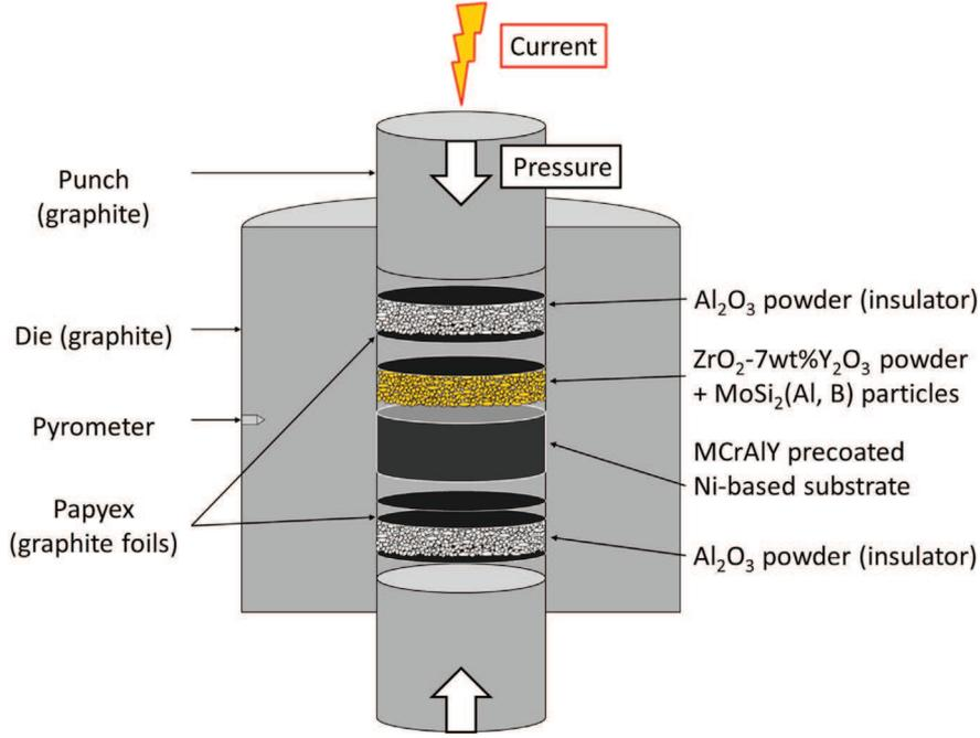
Fig. 1. Schematic arrangement of materials in the graphite die for manufacturing of self-healing TBCs with spark plasma sintering (SPS).
