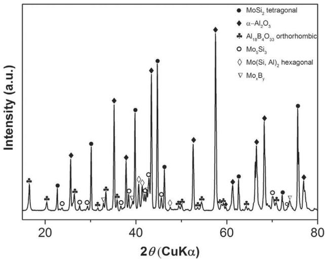
Fig. 2. Diffraction pattern of encapsulated MoSi<sub>2</sub> based particles alloyed with 2 wt% B and 6 wt% Al after annealing at 1200 °C for 1 h in Ar.
