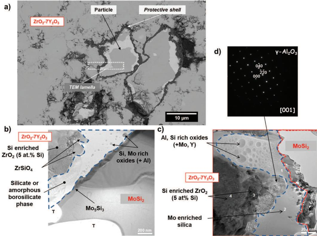
**Fig. 3.** Composite of encapsulated  $\text{MoSi}_2(\text{B})$  based healing particles embedded in YPSZ after annealing in Ar at  $1100\text{ }^\circ\text{C}$  for 24 h: (a) cross-section of the composite just before lift-out of a thin FIB lamella. (b) and (c) TEM images of the FIB lamella after final thinning. (d) diffraction pattern of a  $\gamma\text{-Al}_2\text{O}_3$  crystallite. Here, 'T' denotes some undesirable pores introduced during the thinning process.
