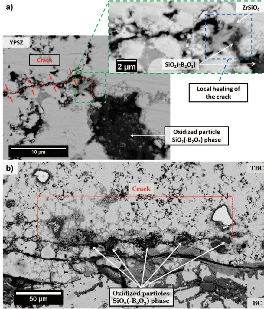
**Fig. 8.** SEM backscatter electron image of a cross-section view of a TBC made of: (a) a mixture of YPSZ and 5 vol% of encapsulated MoSi<sub>2</sub>(B) based particles after 151 cycles of 1 h at 1100 °C, and (b) a mixture of YPSZ powder and 10 vol% encapsulated MoSi<sub>2</sub>(B) based particles sintered on a NiCrAlY coated substrate after 1108 cumulated hot hours at 1100 °C (31 cycles).
