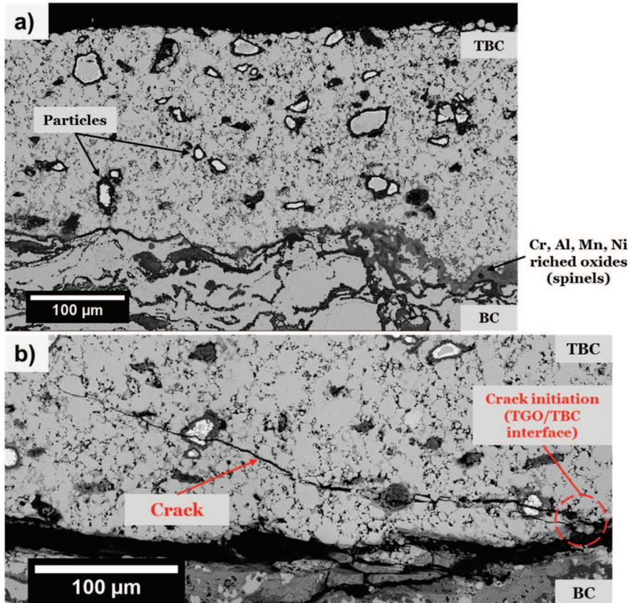
**Fig. 7.** SEM backscattered images of cross-section views of a TBC made of a mixture of YPSZ powder and 10 vol% encapsulated MoSi<sub>2</sub>(B) based particles sintered on a NiCrAlY coated substrate after 1108 cumulated hot hours at 1100 °C (31 cycles): (a) uncracked area, (b) cracked area near the spalled area.
