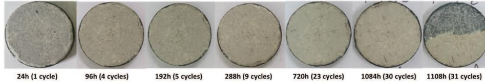
**Fig. 6.** Evolution of damaging during thermal cycling at 1100 °C of a complete self-healing TBC system made by spark plasma sintering of a mixture of YPSZ powder and 10 vol% encapsulated MoSi<sub>2</sub>(B) based particles sintered on a NiCrAlY coated substrate.
