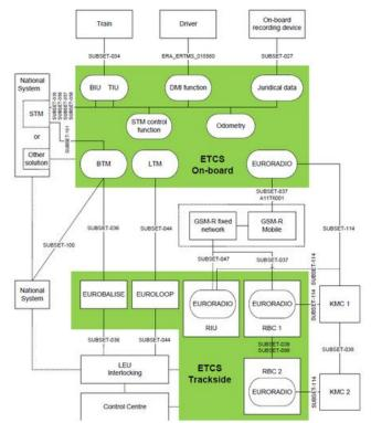
Fig. 1. ERTMS/ETCS system architecture.
