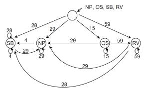
Fig. 6. Finite automaton for the identification of train operations modes.
