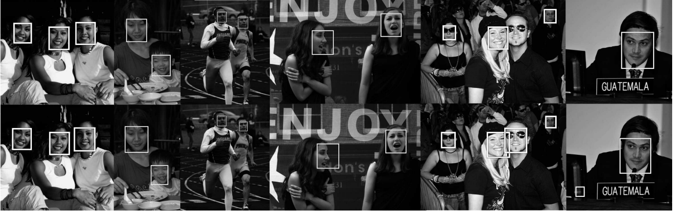
Fig. 3: Some CFF face detection results on the AFW dataset. Top : exact model; bottom : approximation A_{7,3,3,3} . Despite the very coarse approximation, the results are very close. In the second last image, the approximate model even detects an additional face, missed by the original CFF. However, in the last example a false detection is produced.
