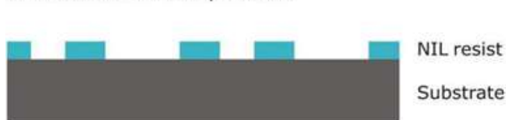
Pattern transfer Step 1: Etch
