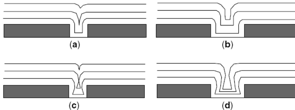
Figure 7.17 (a) Gap filling with conformal step coverage. (b) Conformal deposition of a larger gap with the same process does not lead to gap filling but the original step height remains. (c) Void and (d) cusp are formed when step coverage is maximum at the step corner
