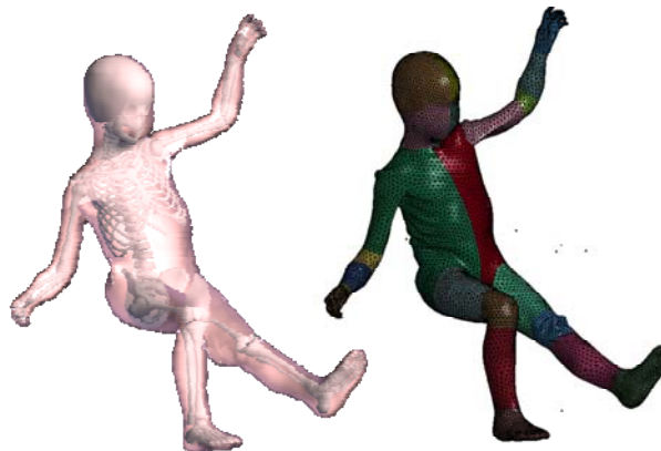
Figure 20: Child model in the PIPER pre-position module (left) and same posture obtained by simulation with the Ls-Dyna solver (right) using PIPER FE input export feature.
