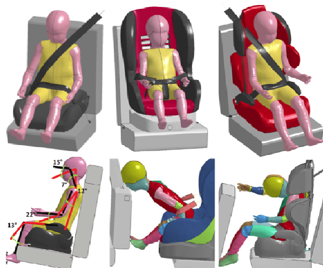
Figure 25: Application with the PIPER child model and the PIPER parametric vehicle environment model: accident reconstructions were performed using physical reconstructions with dummies as a baseline. The model was first scaled and then positioned in PIPER.
