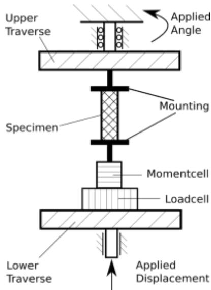
Figure 2- Schematic of the loading and measurement device'
