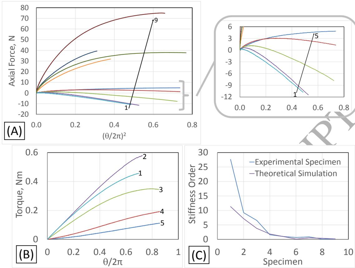
Figure 4- (A) Measured Poynting effect for the 9 specimens. (B) Torque-twist behavior for the specimens 1 through 5 that exhibited widely contrasting Poynting behavior including reversal from positive to negative Poynting effect. It is notable that the volumetric mass density had negligible variation among specimens 1-5. (C) Stiffness order of the 9 specimens calculated by normalizing with the stiffness ratio of specimen 5.
