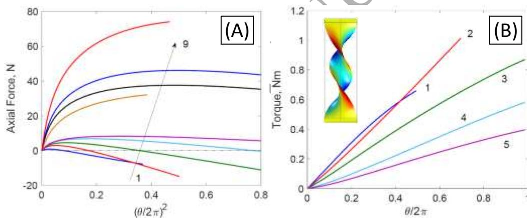
Figure 5- (A) Predicted Poynting effect utilizing a 2<sup>nd</sup> gradient continuum model. (B) Predicted torque-twist behavior for the specimens 1 through 5 that exhibited widely contrasting Poynting behavior including reversal from positive to negative Poynting effect. Inset shows an example simulated deformed configuration at 360°.
