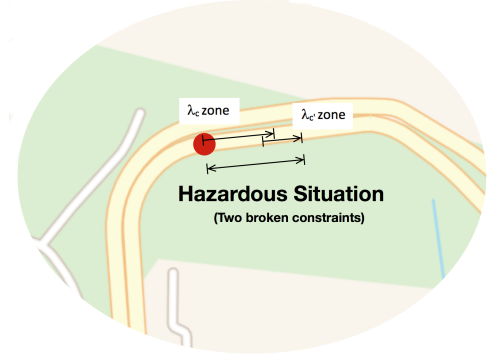
Fig. 3. Distribution of hazardous situations in the navigation map, after multiple trips
